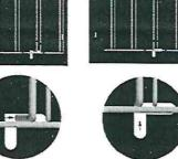
Move the grid in the direction indicated so that moves into the slot along the coast of the oven
